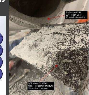
This customer asked if SCP could manufacture a SCProbond<sup>™</sup> N lining for their screw conveyor to keep the flights from losing diameter. We were provided with the dimensions of the both the screw and housing and got to work on these contoured 90 degree flight plates that have extended the conveyor lifetime over 20 months and counting.
